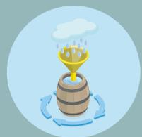
Install a water butt to capture and store rainwater, which can be used for the garden. This reduces the amount of rainwater going into the sewer system, which reduces the risk of flooding.
